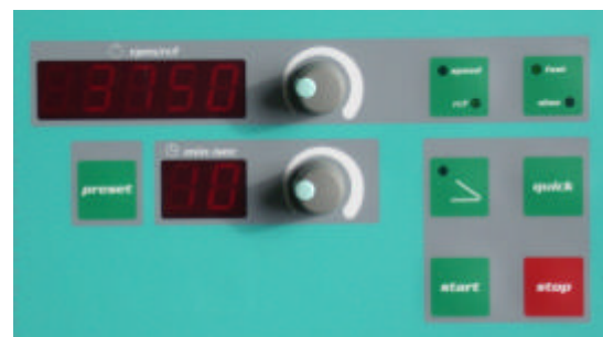
Fig. 8: Centrifuge display – 3750 rpm – 10 min
