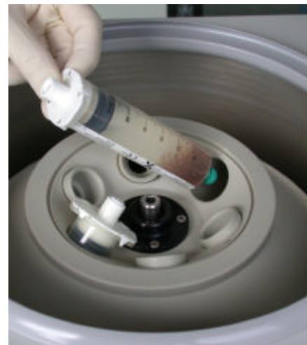
Fig. 7: a balance with water is placed in the centrifuge
